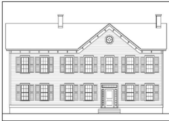
Fig. 16: Improper Addition To Existing Building – This addition blurs the line between the old and the new construction and the original scale and massing of the original design is lost.
