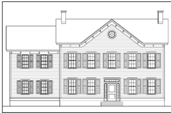
Fig. 15: Proper Addition To Existing Building – This addition preserves the original scale and massing form of the older building, while still appearing to match the original character. The new addition is distinctly separate from the original building, and the line between old and new is visible.
